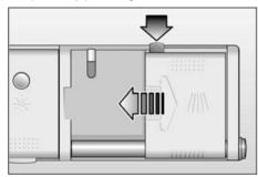
When the door is half open, press the button on the right side of the detergent dispenser. Swivel up the detergent compartment and cover. The detergent compartment can easily be locked into position by lifting it slightly.
